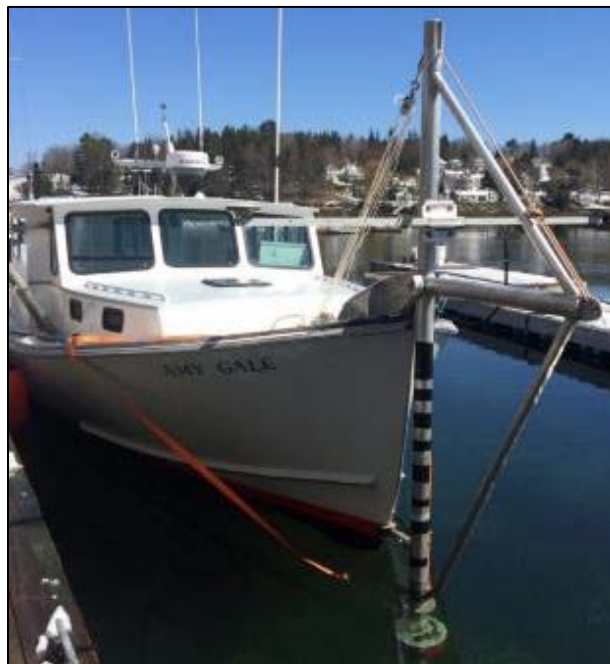
Figure 4 – R/V Amy Gale shown with pole-mounted dual GPS antennas, Kongsberg EM2040C multibeam sonar, MRU (not visible), and surface sound speed probe (not visible) in acquisition mode
